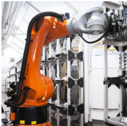
Linkage of four machining centers with KR FORTEC Foundry
