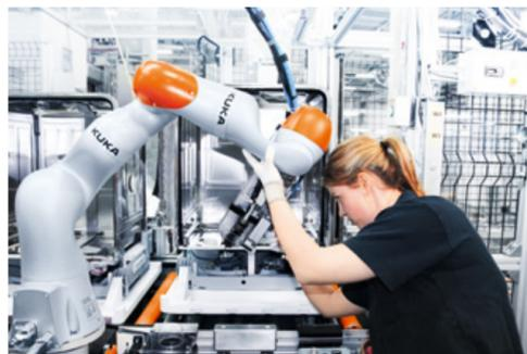
Efficiently fasten screws in dishwashers using the sensitive colleague.
