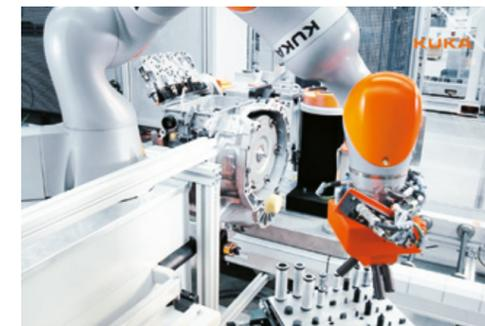
The LBR iiwa inserts sealing sleeves with fine control and a high degree of precision.
